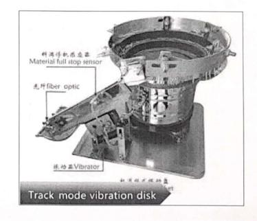
Therearetwomaincountingmodesofvibrationdisc, trackmode, boxmode and belt linemode. Trackmode: mainly used for screw products; This equipmet is equipped with a 620 mms crew plate; Boxmode: mainly used for granular products, such as gaskets, nuts, etc.
