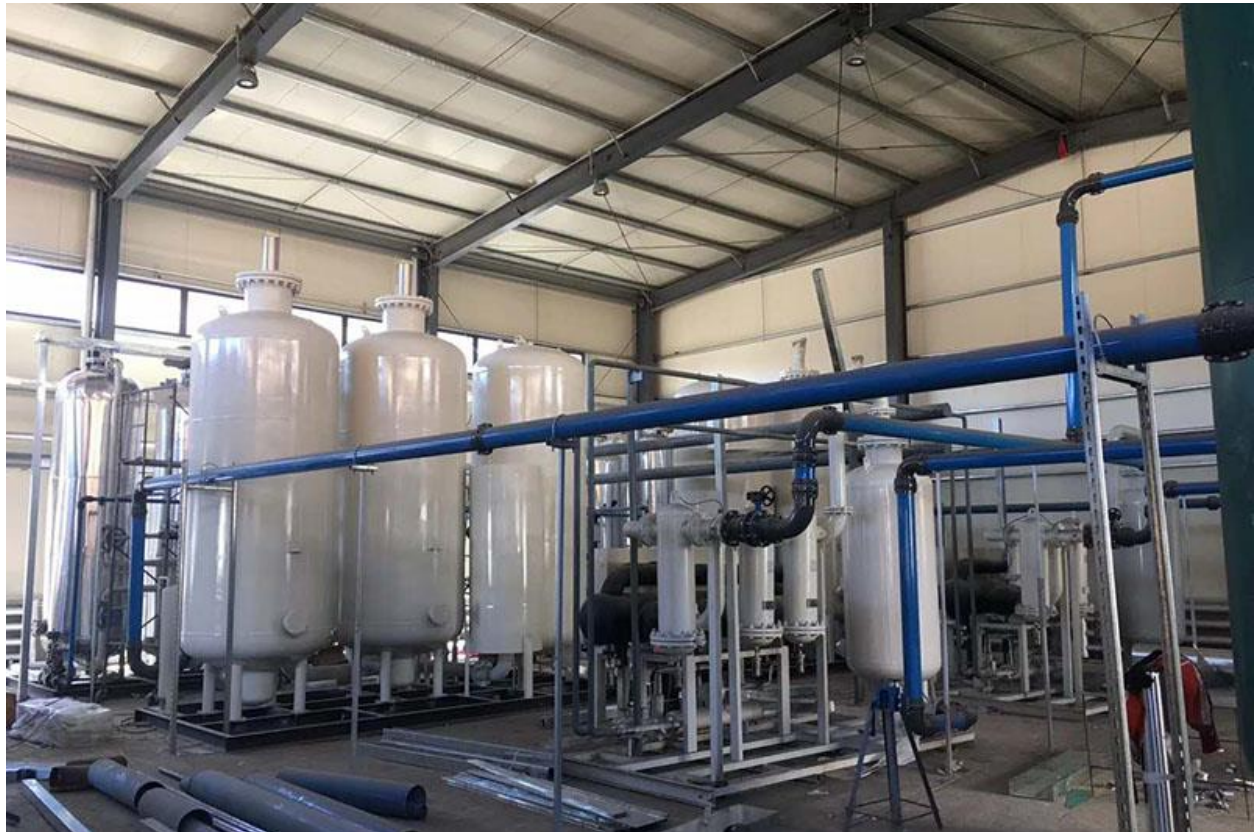
20L/h Small Liquid Nitrogen Generator
