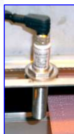
Upper belt tracking by ultrasonic sensor
