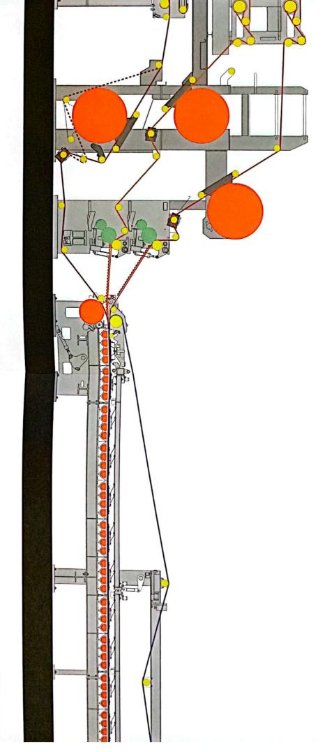
Automatic shoe pressure control with zero edge crush
