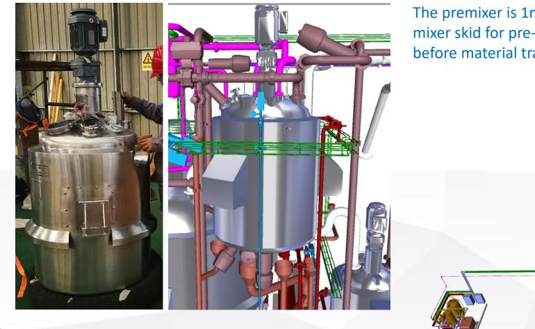
The premixer is 1m3 integrated into main mixer skid for pre-heating & mixing before material transferred to main mixer
