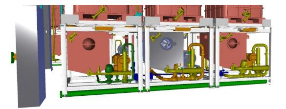
IBC stations are used for storing raw materials. They are made of SS316L, added to the mixer for circulation as well.
