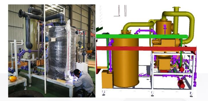
HCL bulk tank is connected with main mixer skid to supply raw materials. Scrubber is integrated with tank skid for the purpose of health & environmental protection.
