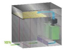
Down flow booth is used for Enzyme transferred from IBC to mixer. In the DFB, the air is filtered to provide the operator a safe working room.
