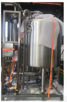
The CIP skid is composed of balance tank, CIP supply pump, dosing pump, Heat exchange, valves and piping. After each batch, the process line will be cleaned with hot/cold process water to avoid contamination before next batch.
