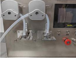
2: After installing the filling nozzle, note that the end of the filling nozzle is about equal to the bottom line of the magnet
