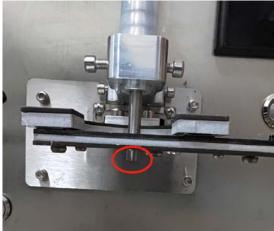
3: Move the bottle clamp to ensure that the filling nozzle is concentric with the bottle mouth, and the filling nozzle must not collide with the bottle mouth.
