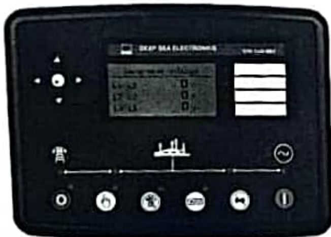
Control Panel: Deepsea DSE7320
