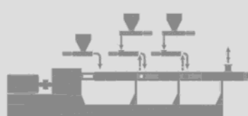
Filling and Reinforcing
