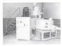
Material of the Container: 1Cr18Ni9Ti, Stainless steel, inner surface is very utmost smooth and stiff, featuring wear-resistance and corrosion resistance, material will not sticky to the container.
