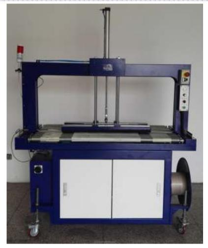
Automatic high-table pressurized strapping machine is a automatic pressure for loose items packaging operations, the up and down movement of the machine by the cylinder to realize the compression of the item at the same time of compression will be automatic strapping machine, thus will decrease the volume of goods, so as to reduce the cost during the transit. The machine has high-table and low-table models.
