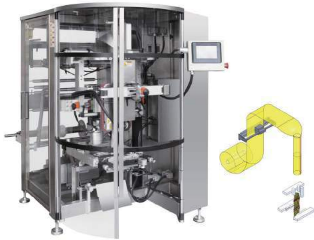
背封连续式立式机 BACK SEALED, CONTINUOUS MACHINE
