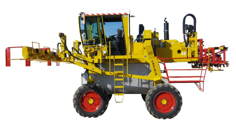
A self propelled machine on 4 driving wheels with hydrostatic traction provided by engines "Poclain" on wheels.
