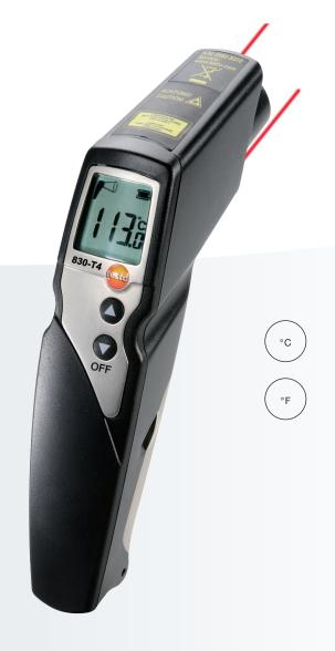
The testo 830 non-contact infrared thermometer family is used to measure surface temperatures across a wide range of applications from the HVAC, refrigerated warehousing, transport of pahamaceuticals, to food, food service and spot checking of perishable goods. The testo 830 is used in supermarkets to check open shelf refrigerated coolers as well as by car mechanics to check the transmission fluid's temperature to assure the right filling level.
