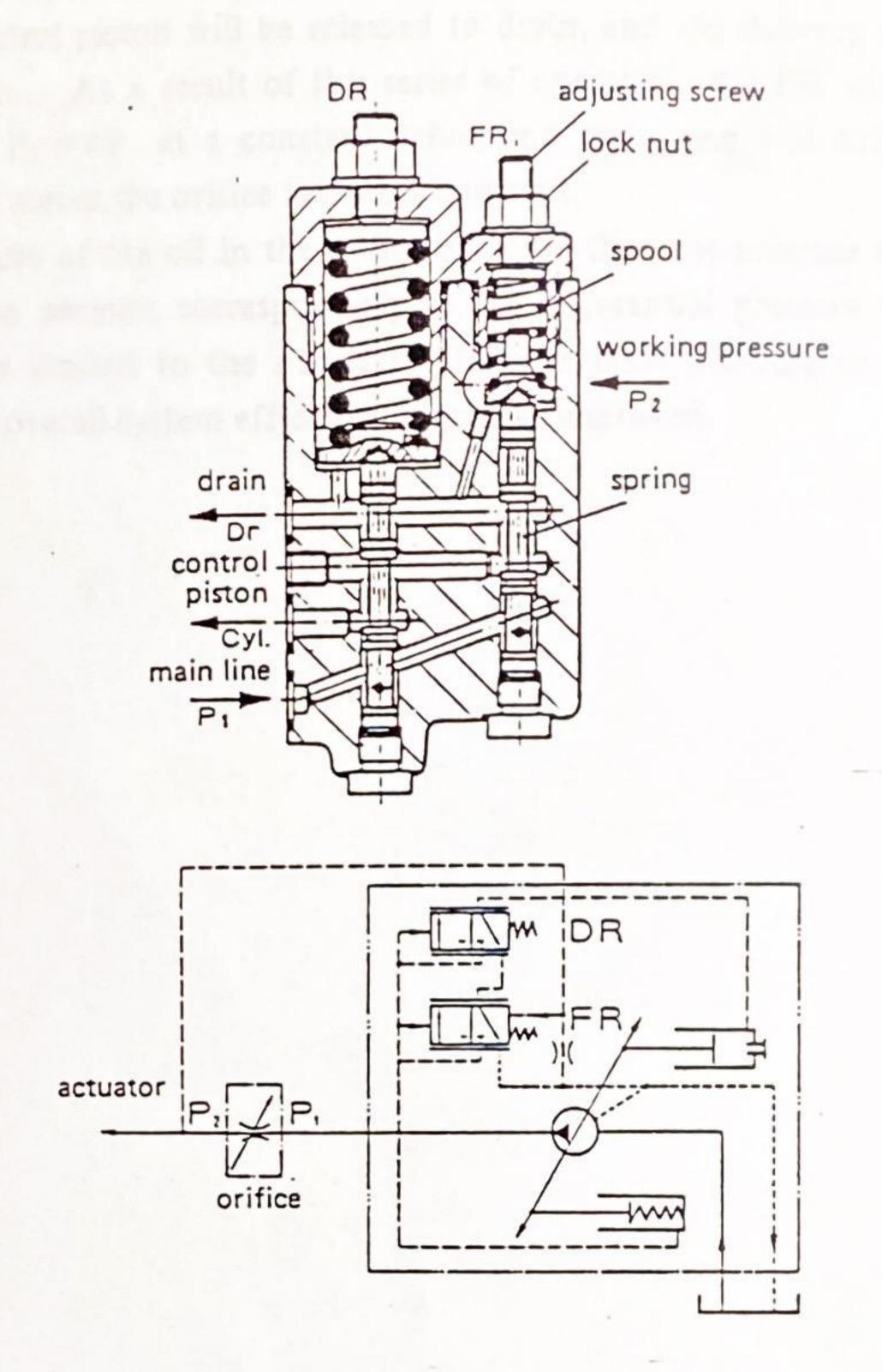
A variable or fixed orifice is installed in the main line, and the pressure difference across the orifice mainteined constant, that is, the delivery flow is maintained constant.
