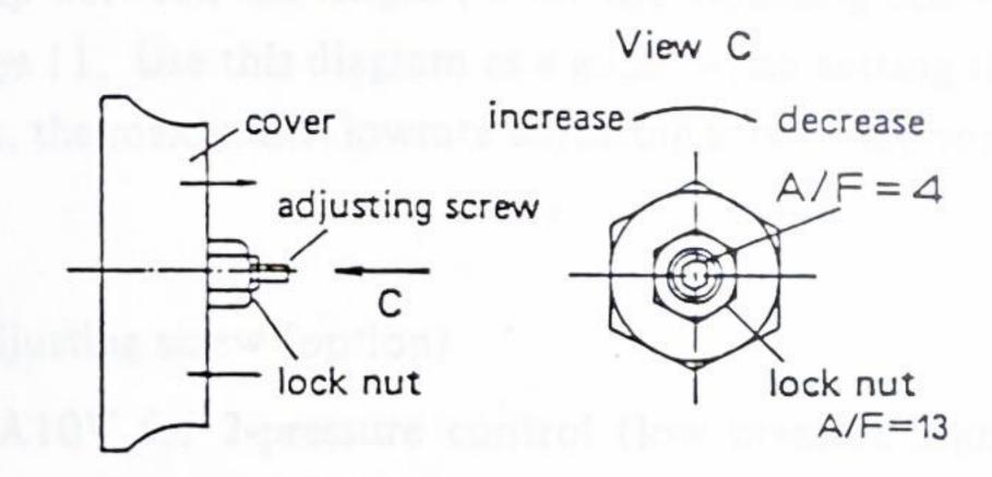
\* The installation position of the maximum flowrate adjusting screw and the DR (DFR) valve differ, as shown in the drawing, depending upon the direction of rotation of the pump.
