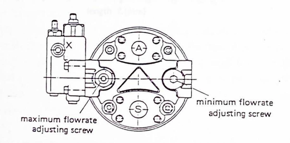
\* The relationship between the length (2) of the screw and the flowrate is as shown in the diagram below. Use the dotted lines in this diagram as a guide when adjusting the flowrate.
