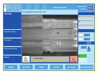
Automatic scanning of the entire length of the U-tube is possible as well as manually controlled viewing positions. The video clarity, magnification, and resolution is the very best available. Rudolph's exclusive VideoView™ is protected under Patent #7,437,909.
