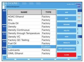
For unique measurement applications, create a sample method using an unlimited number of Concentration Tables, Formulas, and Polynomials to match the measurement methods used in your laboratory. A few customized sample methods shown below:
