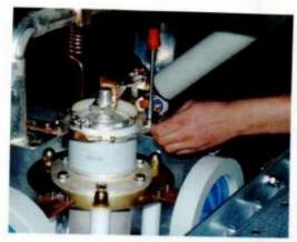
Unscrew the 7 mm nut that tight the grid-cathode capacitor
