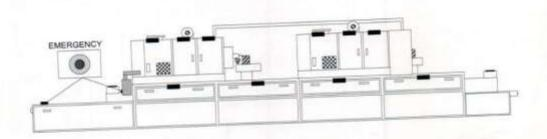
The diagram shows the emergency pushbuttons on the machine and on the control panel. The safety microswitches are also shown.
