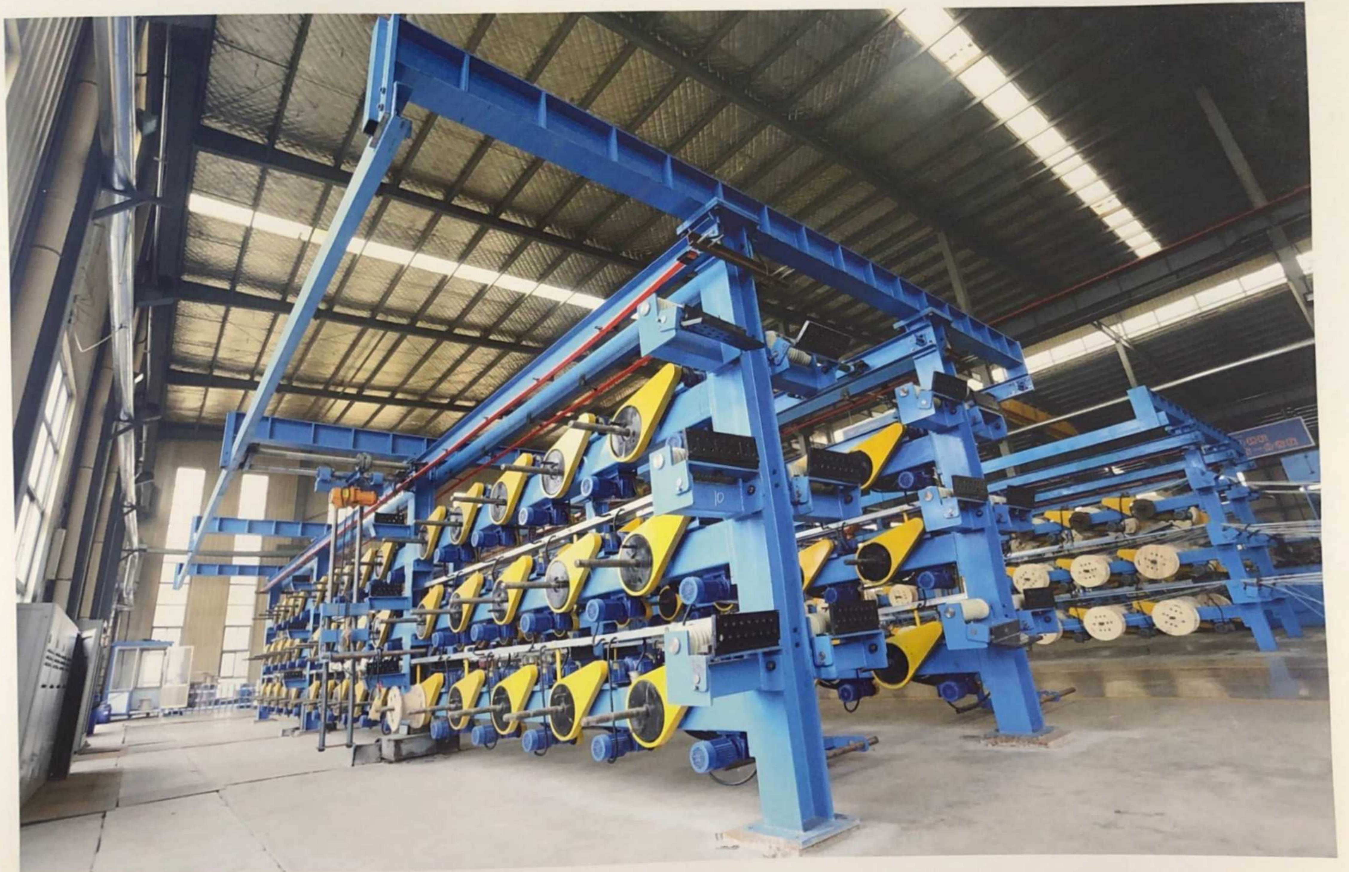
高耐磨自润滑陶瓷钢丝变位导向装置 The steel cord guiding and displacement device made by ceramic has the function of high wear resistant and self lubricating.
