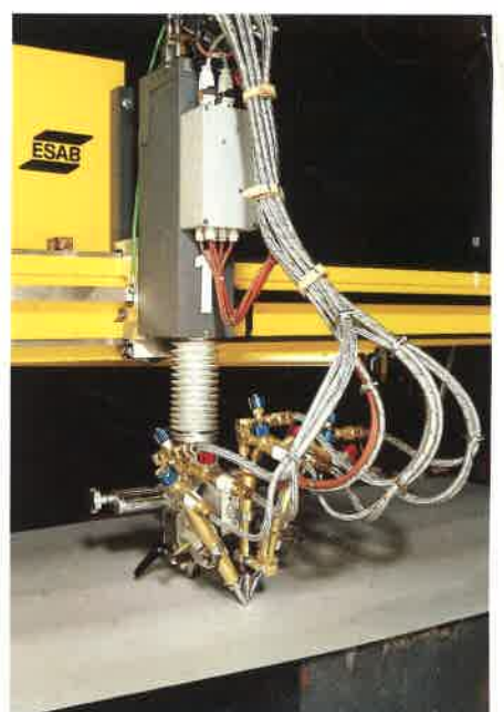
Torch carriage B1 with height adjustment and triple nozzle burner arrangement (±90°)
