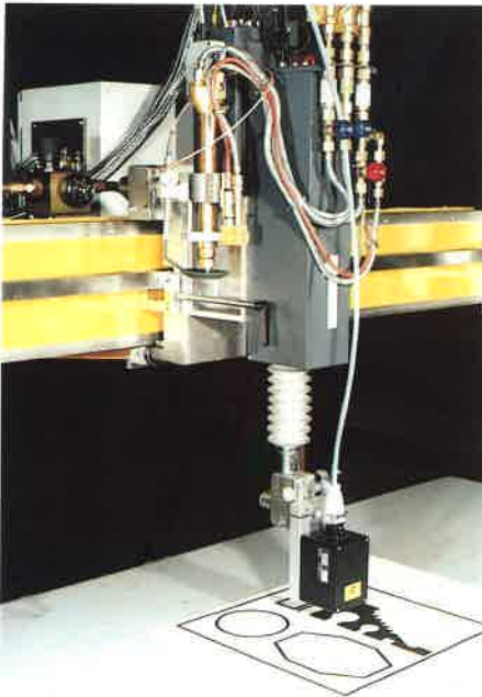
Torch carriage A2 with exchange unit for Teach-Trace and oxy-fuel equipment
