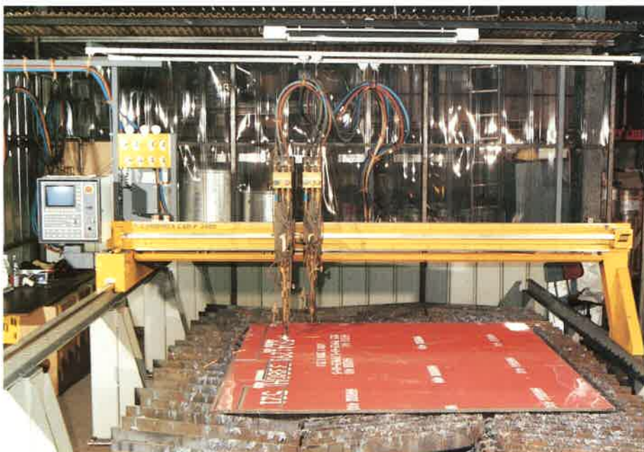
COMBIREX CXD-P equipped with NCE 390 and two torches for oxy-fuel cutting
