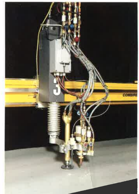
Torch carriage B1 with motorized, capacitive height adjustment and powder marking device
