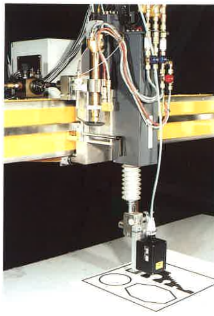
Torch carriage A2 with exchange unit for Teach-Trace and oxy-fuel equipment
