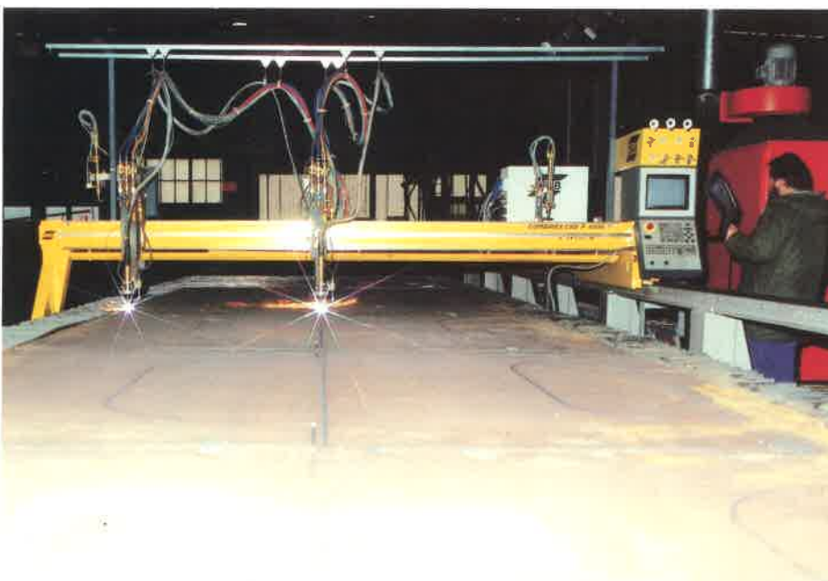
COMBIREX CXD-P equipped with NCE 510 and two exchange units for plasma/oxy-fuel cutting
