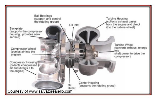
**The compressor** is spun by the rotational force created by exhaust gases flowing through the turbine. This would feed the intake side of the motor. Air is inducted into the compressor and then compressed into the piping, feeding the air intake ports of the motor. This creates an increased flow, as well as density, of air to be fed into the combustion chambers of the motor.
