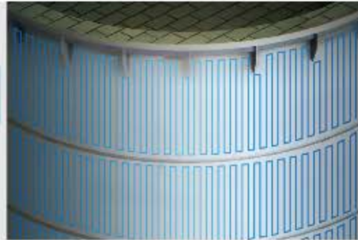
Furnace shell coil water cooling system
