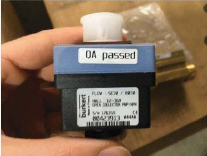
During visual inspection of the electronic device of the flow sensor
