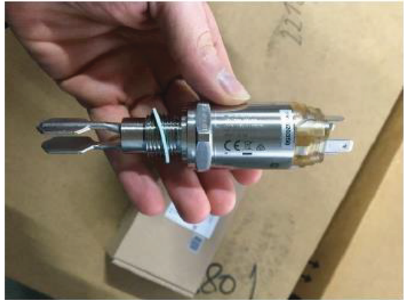
During visual inspection of the level limit switch
