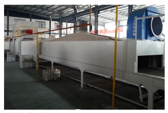
Desktop drying furnace: electric power: 16.5KW
