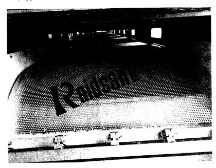
a. Dimension:  $47140 \ (\pm 50) \times 1500 \ (\pm 1.0) \times 1.0 \ (\pm 0.1) \ \text{mm} \ (\text{length} \times \text{width} \times \text{thickness})$  Imported special steel belt, there are NBR strips at both sides of steel belt's back for avoiding belt's deviation.
