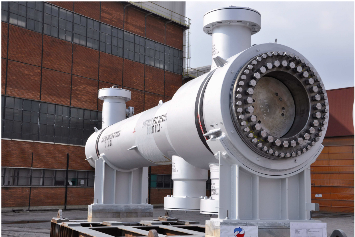
Figura 1: Threaded Closure HE delivered for a Refinery Conversion Project in Portugal
