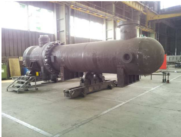
Figura 5: Threaded Closure Heat Exchanger with tubesheet designed at full pressure.
