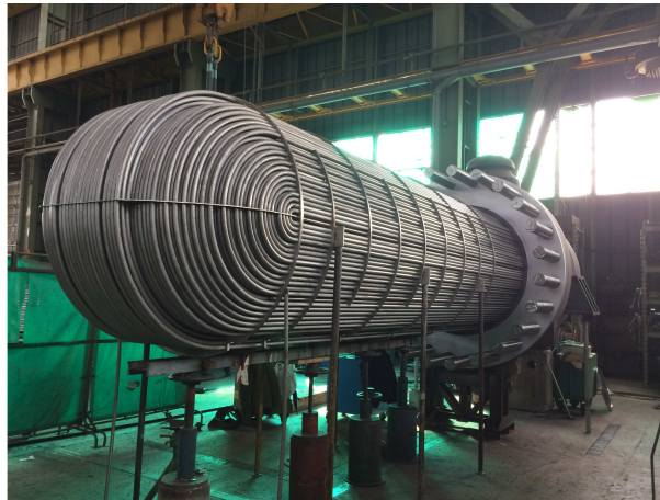
Figura 4: Tube bundle of Threaded Closure Heat Exchanger with tubesheet designed at full pressure.
