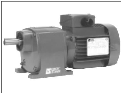
Compabloc 1000 geared motors with parallel gears are used to adapt the speed of the electric motor to that of the driven machine. Their size is therefore determined by the motor power ( $P$ ) expressed in kilowatts (kW) and the output rotation speed of the gearbox ( $n_S$ ) in revolutions per minute ( $\text{min}^{-1}$ ). The main characteristic of the speed reducer is the nominal output torque ( $M_{nS}$ ) expressed in Newton-metres (N.m).
