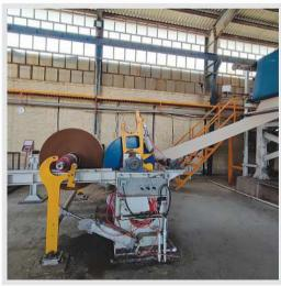
rewinder is used for slitting & rewinding paper
