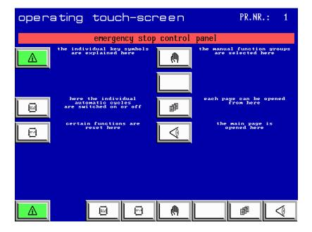
This image appears after the machine has been switched on. It shows a survey of all the symbols used for the buttons (bottom bar) including explanation.
