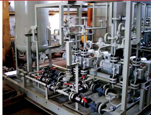
Plant South Pars Phase 6 EPC STATOIL Item Chemical Injection Package Material SA516/SS316L/S235 QTY 21
