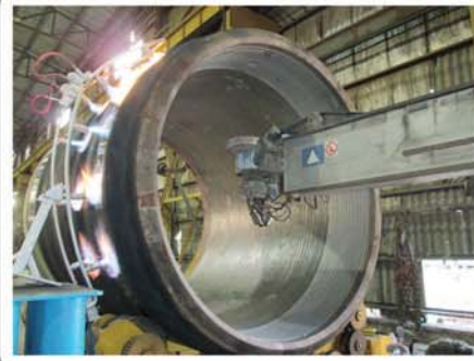
Weld Overlay : Column & Boom (Shell Cladding Column & Boom - Rotator) Weld Overlay
