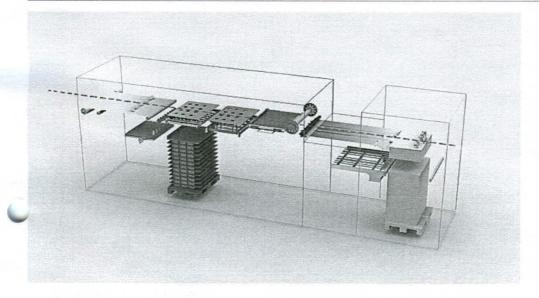
A flat bed die-cutting press may be an offline, stand-alone machine, or may be inline with a printing press and/or other units. Having been fed into the press and held by a gripper bar, the sheet of substrate is transported through a number of stations which carry out sequential processes. The exact configuration of a flat bed die-cutter will vary depending on the application but, in broad terms, the elements that may be present are:
