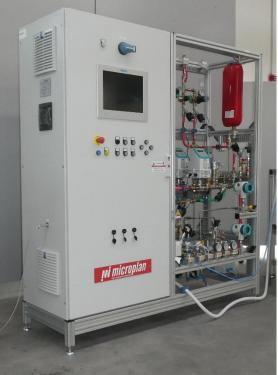
NOTE4: the offered test bench includes the DI and DO signals intended for the connection of the bench to the electrical safety test station. They are the same channels that were included in the test benches of the B310 series for that purpose and they can be recognized in the I/O channels table reported in Annex A.
