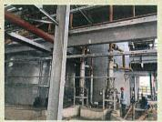
Raw material includes granulated fiber, starch and so on, all the material and additive will form the slurry with certain concentration by conveying, mixing and stirring. The slurry will be pumped into high level tank and fed to net in the shape of overflow type.
