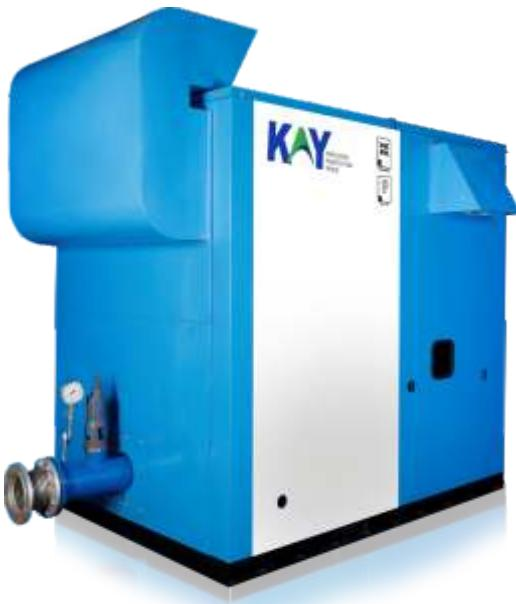
Acoustic hood covers the complete blower and motor arrangement. Its soundproof cabin decreases the overall sound of the system to the accepted norms as per IS specifications. Provision of exhaust fan decreases heat in the chamber and fixing of the anchor bolts results in rigid base to the acoustic hood. This is a very effective enclosure to provide noise reduction of 15 to 20 dBA or more, to comply with international noise levels. It is also available for all blowers and models.
