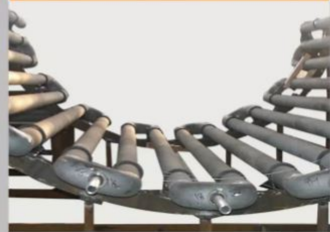
Overheat steam furnace tube
