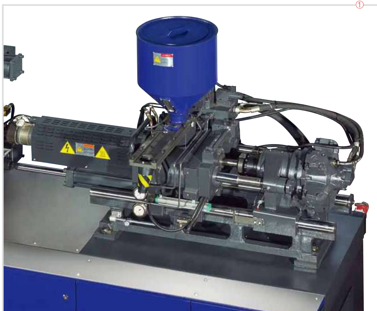
Figure ① The rigid one piece injection base supports the common slide rail for injection and screw movements, reducing stress and increasing movement precision. The balanced twin injection cylinders apply equal force to the screw during injection.
