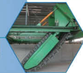
Turning unit lifted by hydraulic system.
