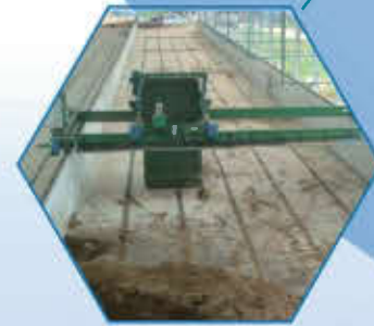
Longitudinal and lateral movement of turning unit for working in any position.
