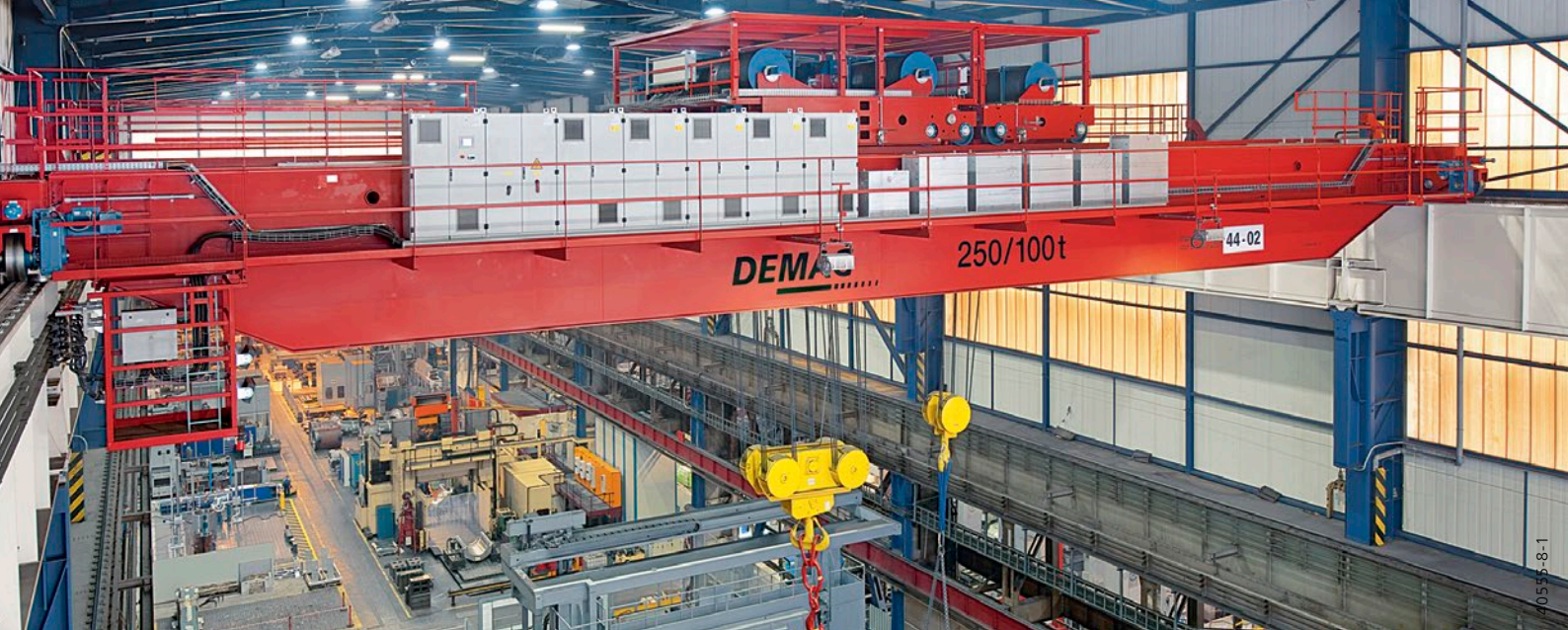
Process crane equipped with a 250-tonne MPW double hoist unit on a crab and a 100-tonne MPW open winch unit
