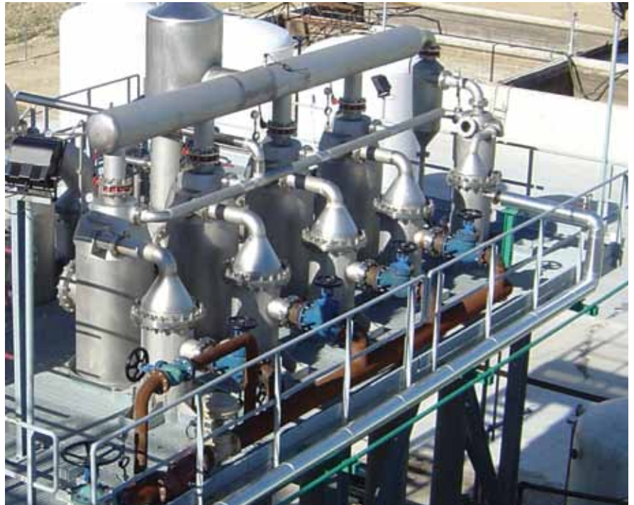
➤ HRS Unicis Series scraped-surface evaporators are used to maintain thermal efficiency and remove fouling during evaporation in ZLD installations. Image courtesy of HRS Heat Exchangers.
