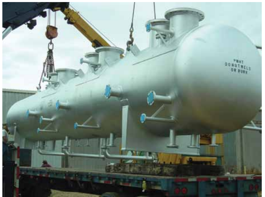
≈ Horizontal mixing vessel - carbon steel with PWHT and high-temp coating
