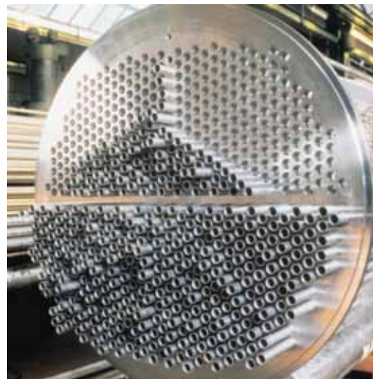
≈ Heat exchanger assembly.
