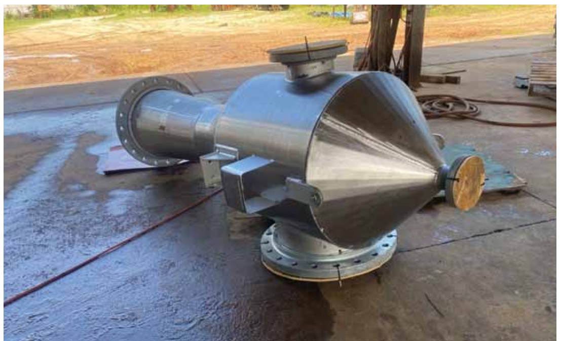
➤ Eductor for a chemical manufacturer, used in a carbon capture process at the plant. It is made of Hastelloy C276.
