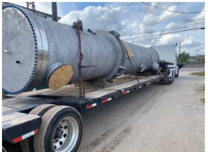
⌚ Vertical NEN style turpentine condenser rebuilt in 4 weeks (all 304L SS).
