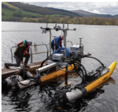
The photo of the OPT Wave Adaptive Modular Vehicle (WAMV-16) was taken at the end of April 2023 at Loch Ness, Scotland, during trials on the loch to scan it using the UXO detecting technology.
