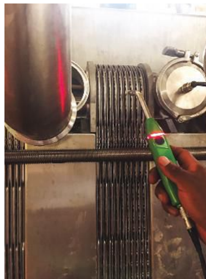
IMAGE 2: The integrity testing precision sensor can identify the type of defect from micro-crack to corrosion, gasket failure and more.
