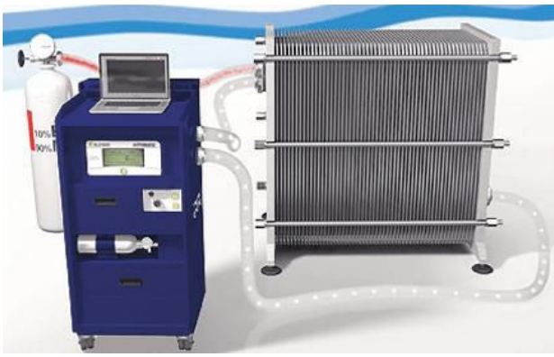
IMAGE 3: Alfa Laval Integrity Tester: Integrity testing uses a mix of hydrogen and nitrogen pumped through the gasketed plate heat exchanger to reveal any microscopic cracks, corrosion or material fatigue.
