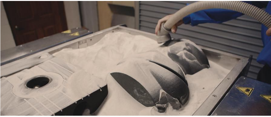
IMAGE 3: Creating new components using a 3D sand printing process
