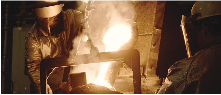
IMAGE 4: An in-house foundry is central to creating new parts and pouring numerous different alloys for castings.
