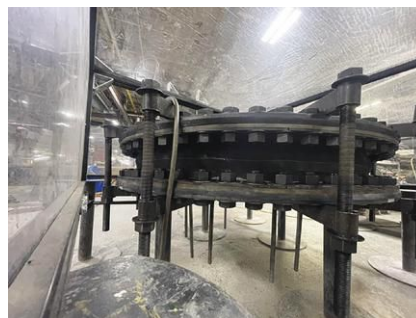
IMAGE 3: 72-inch performance expansion joint during burst testing
