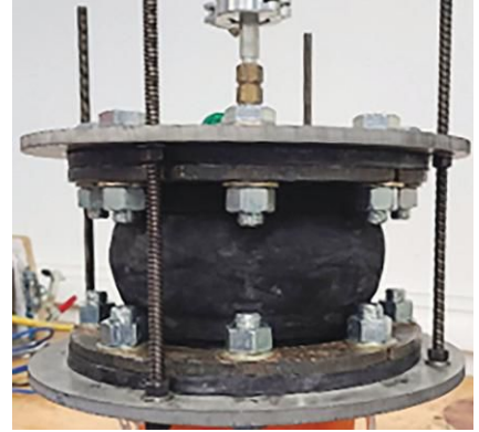
IMAGE 5: Vacuum test at neutral state
