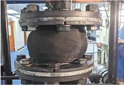
IMAGE 7: Laterally displaced joint for movement testing
