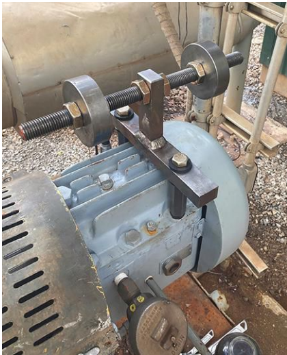
IMAGE 3: Dynamic vibration absorber with two masses
