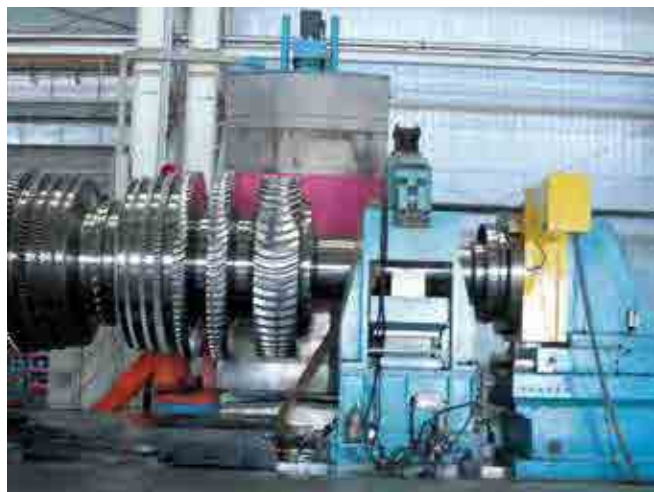
Indexing of the turbine shaft
