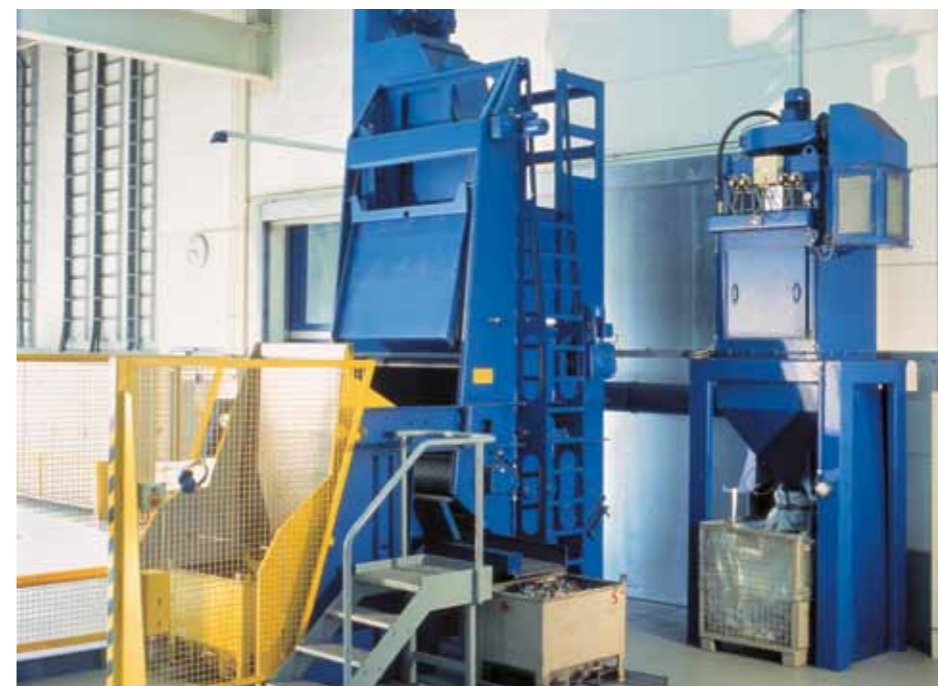
Wheelabrator tumbblast machines are proven in hundreds of applications, for desanding, descaling, shot peening
