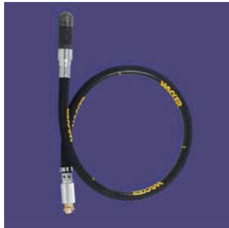
Immersion bottle vibrator: Following diameter are available: 35 mm / 55 mm The immersion vibrator is working with 6 bar air pressure
