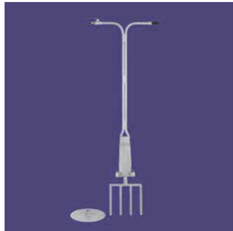
Compressed air vibrator: This device is operated by a ball air vibrator with high frequency and can be used with a fork and with a base plate. The vibrator is operated by hand and is especially suitable for ramming dry refractories which must be filled in layers of 100-120 mm.
