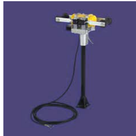
Electric vibrator: The electric vibrator is a hand-operated vibrator, too. The vibration effect is transmitted onto a rectangular base plate via a tube. This tool is especially suitable for small furnaces and for ramming neutral and basic dry linings. Here, the filled layers must not be higher than 60 mm.
