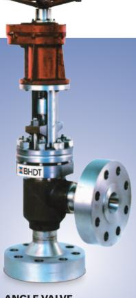
ANGLE VALVE stub ends, steam jacket NS 5", PN 18.5 MPa SA182 F316LUG (Böhler A220)
