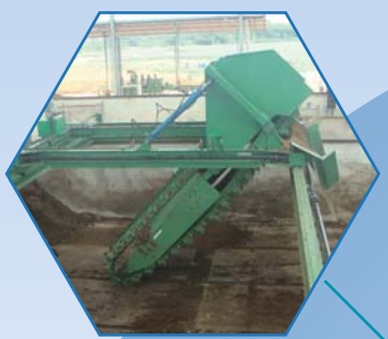
具有对物料翻抛、提升和位移功能,适合深槽作业 Suitable for deep channel for it's turning, lifting and moving ability of materials.
