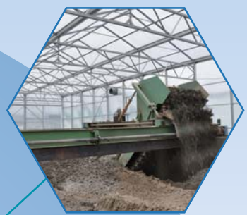
链板长4米,物料在托料板上停留时间长,高位抛散接触空气充分,易降水充氧 Long inclined-conveyor for better oxygenating, and dewatering .
