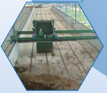
纵向和横向移位可实现槽内任意位置翻抛作业,机动灵活。 Longitudinal and lateral movement of turning unit for working in any position.
