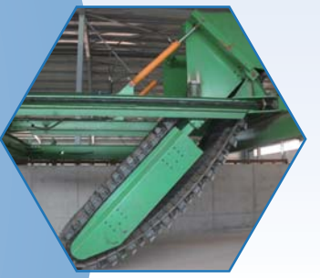
翻抛工作部件的升降采用液压系统操控,柔性工作安全快捷 Turning unit lifted by hydraulic system.
