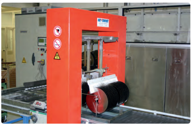
Low-frequency demagnetization tunnel for the demagnetization of saw blades.
