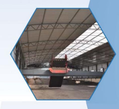
Fermentation channel width up to 20 m for saving construction cost .
