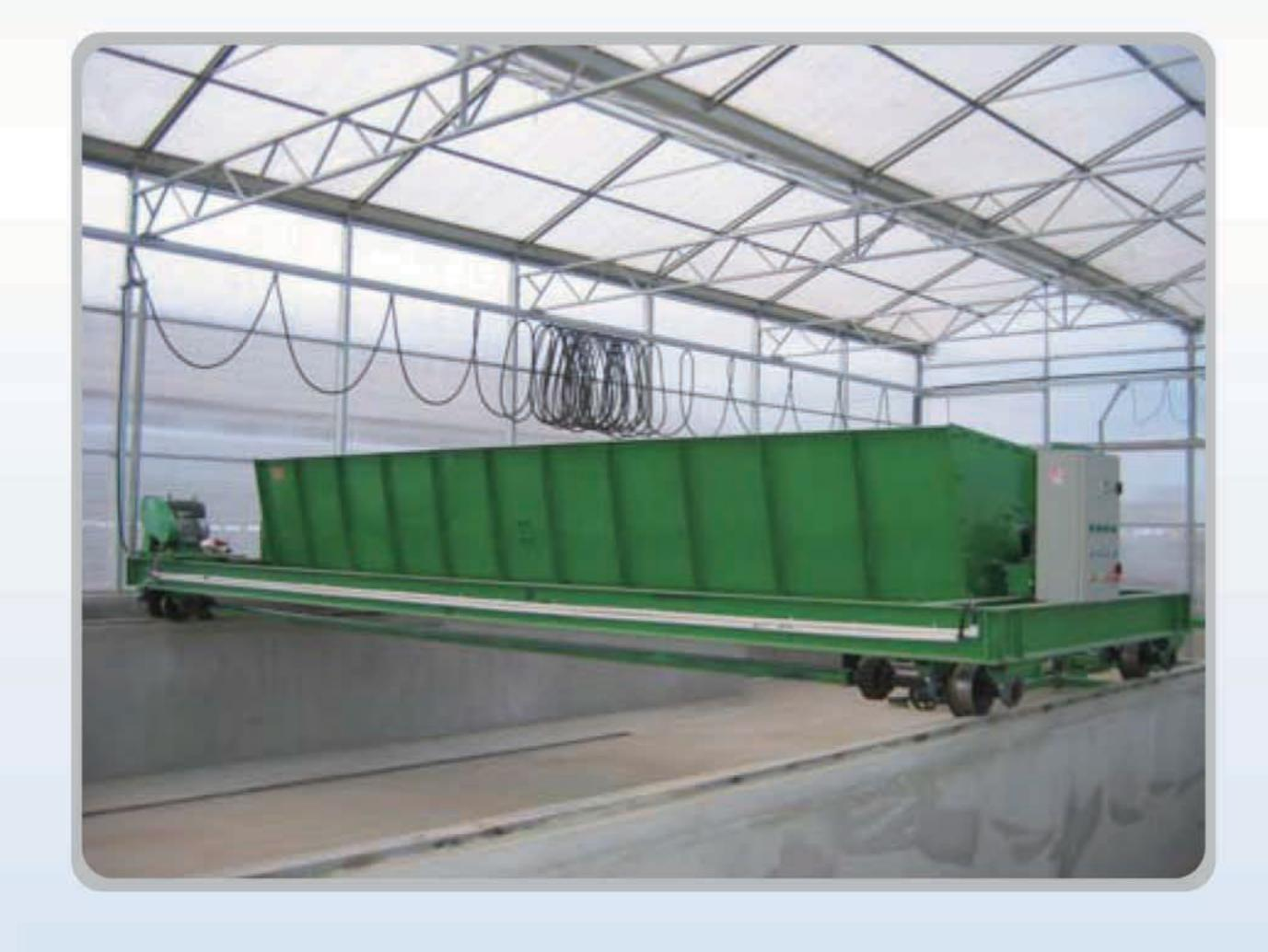
**Application:** Spreading the raw materials along the compost channel to any position with adjustable material layer thickness.
