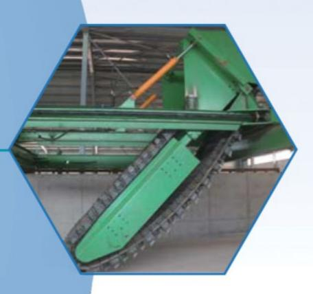
Turning unit lifted by hydraulic system.
