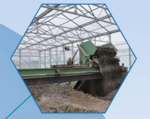
Long inclined-conveyor for better oxygenating, and dewatering.
