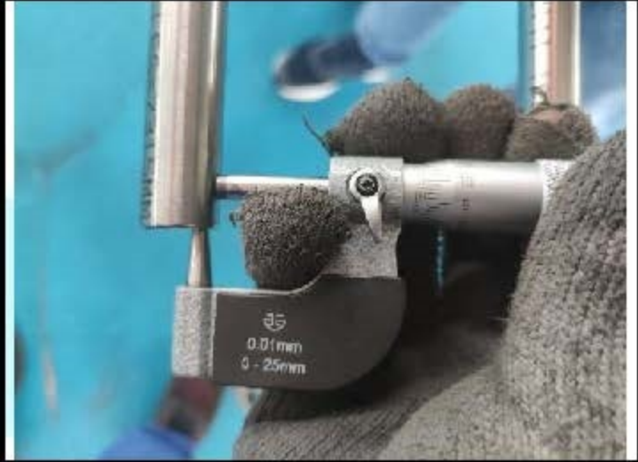
10- Wall thickness inspection
