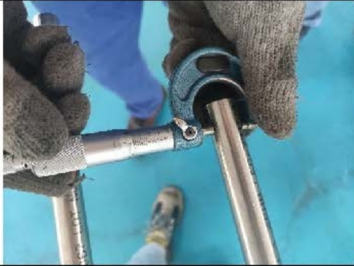
9- Outer diameter inspection
