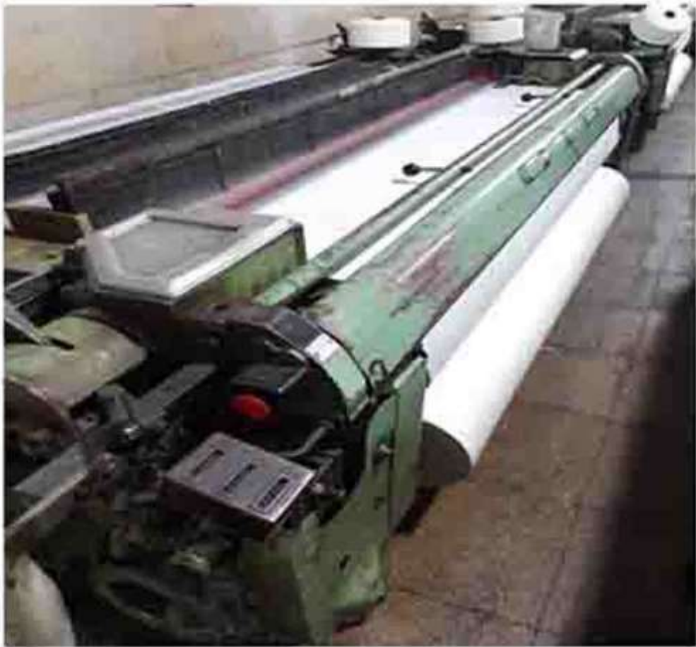
STB 2-180 knitting machine (3500mmx1875mmx1400mm) Fabric bed weaver size 1800mm Year:1993
