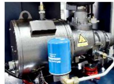
IE4 permanent magnet variable frequency super efficient motor
